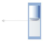
liquid that remains on the pipette walls and in the jet is not included to the measured volume. The pipettes adjusted to the delivered capacity are marked on a label by the letters "Ex".
